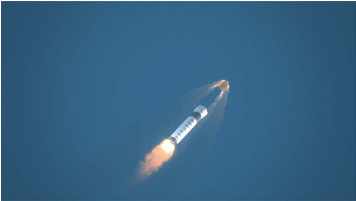
Artists image of the newly proposed launch escape system for the Dragon. The new launch abort system provides crew with emergency escape capability throughout the entire flight and returns with the spacecraft, allowing for easy reuse and radical reductions in the cost of space transport. Credit: SpaceX
