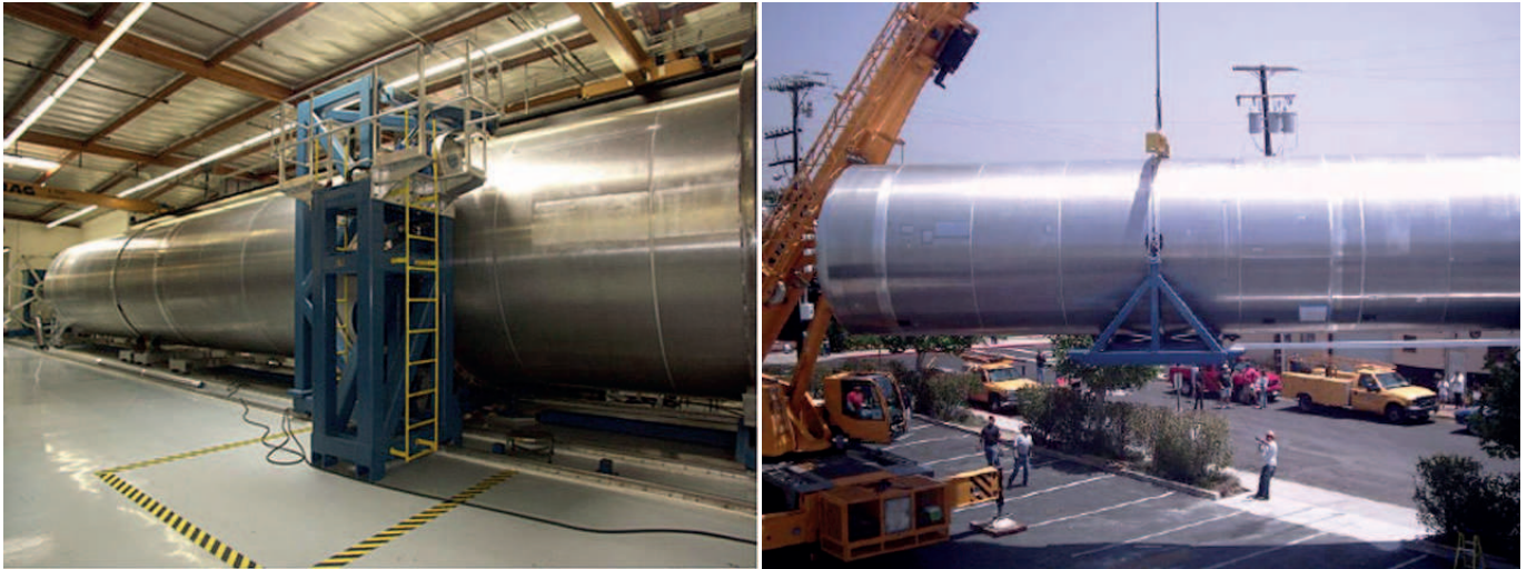
Falcon 9 First Stage on the production line; Moving the First Stage Tank from the manufacturing line to the road.
